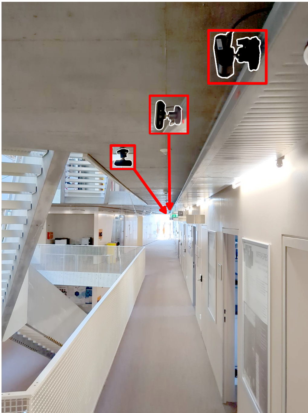
Figure 8.2: Physical setup of the hallway experiment. The corridor is monitored by three strategically placed 4k cameras, ensuring comprehensive coverage of the entire space. This arrangement allows for high-resolution observation and data collection across the length of the hallway.
